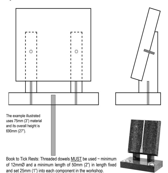
Tick Rests to base: Dowels 16mmØ x 150mm (6") and a maximum clearance of 4mm in the tick rest's dowel holes and 8mm in base's dowel holes must be maintained.
