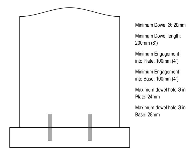
In all cases, a maximum clearance of 4mm in memorial plate dowel hole and 8mm in base must be maintained. Larger diameter dowels can be used to achieve this. This applies to Fig 1, Fig 2 and Fig 3
