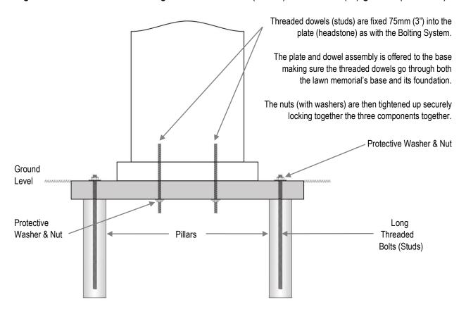
Fig 11 ~ A typical Canopy Set fixed using dowels, locating pegs and ground anchor
