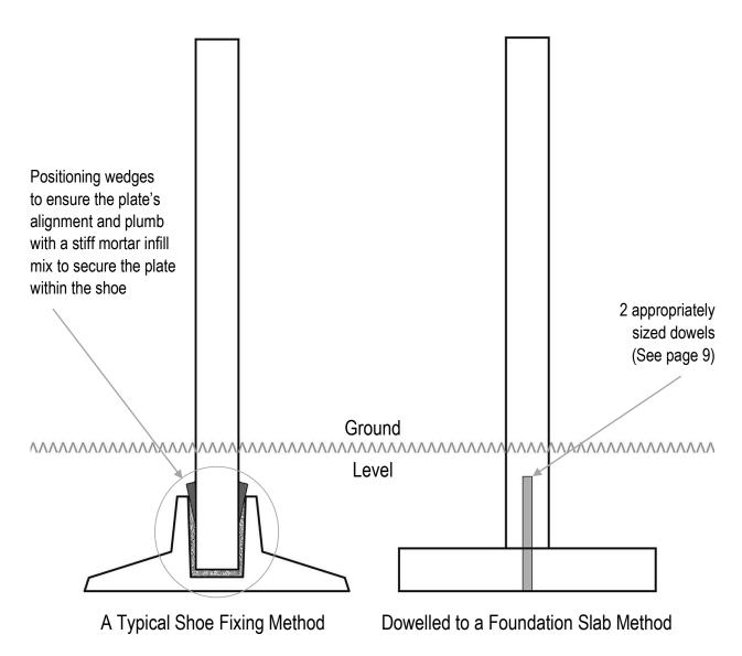
The minimum depth below ground is 375mm (15") or 25% of the overall height (including the foundation) whichever is greater.
