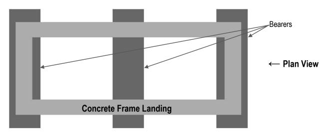
2) A typical corner pillar foundation example: In this case the pillars are made from dowelled 75mm x 225mm x 225mm (3" x 9" x 9") centre dowelled, concrete blocks.
